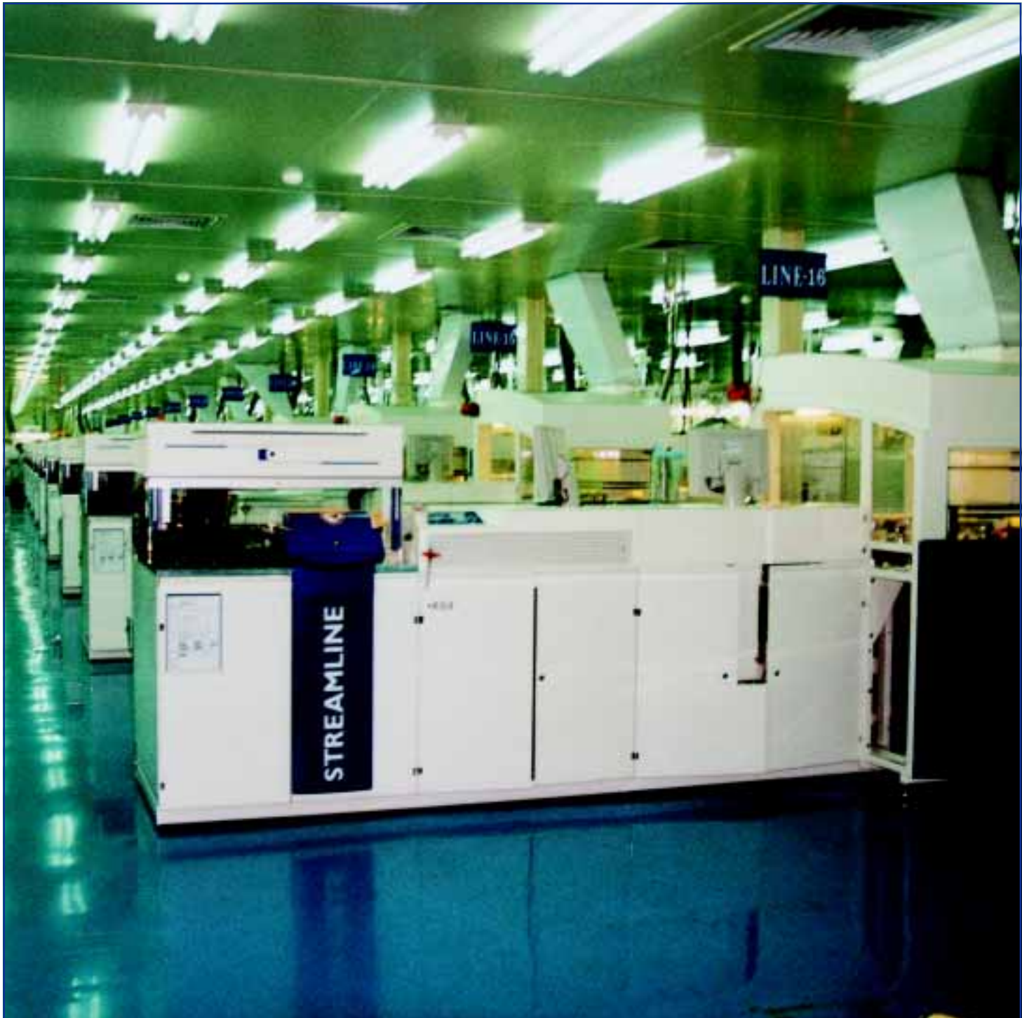
16 STREAMLINE REPLICATION LINES AT A CUSTOMER IN TAIWAN RIGHT PICTURE: DYE-COATING FOR CD-R
