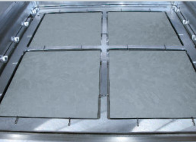
Substrate Carrier with four Si Solar Cells
