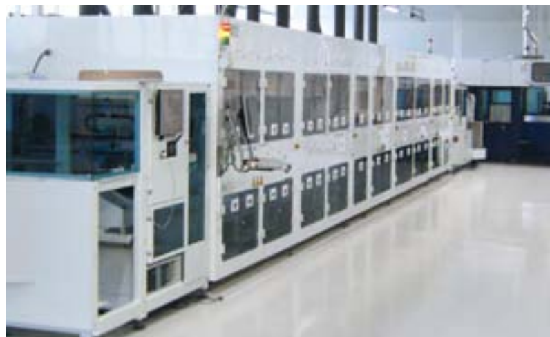
So-called front-end system for silicium solar technology with a handling system, LINEA PSG-Wet Process Equipment plus a SINGULAR AR-coating system
