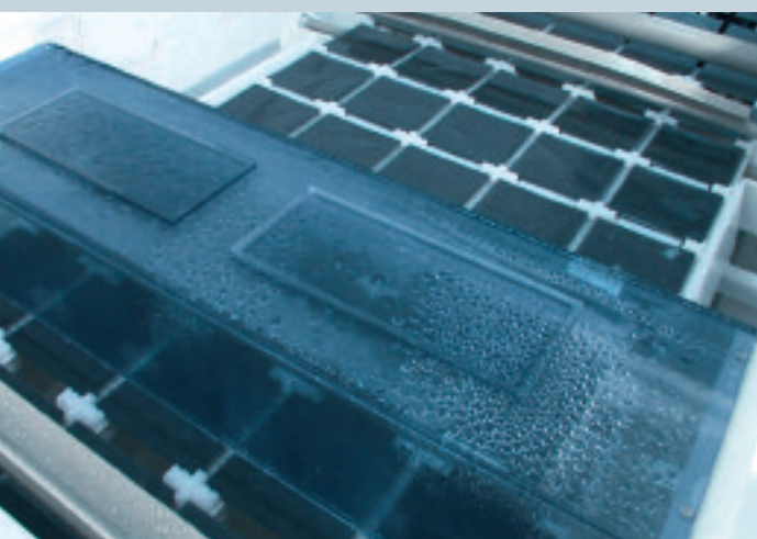
Inner view LINEA with conveyor system for 5 silicon solar cells each
