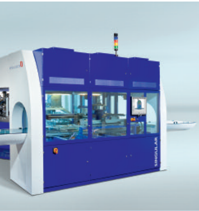
SINGULAR – New production system for silicon solar cells
