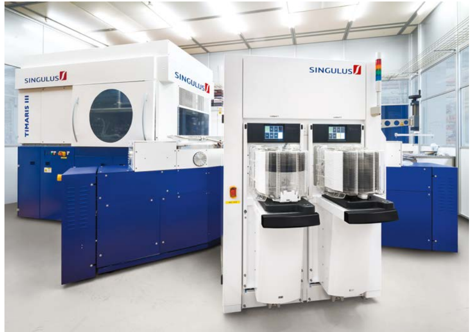
TIMARIS III – Vacuum deposition system for manufacturing of 300 mm semiconductor silicon wafer.
