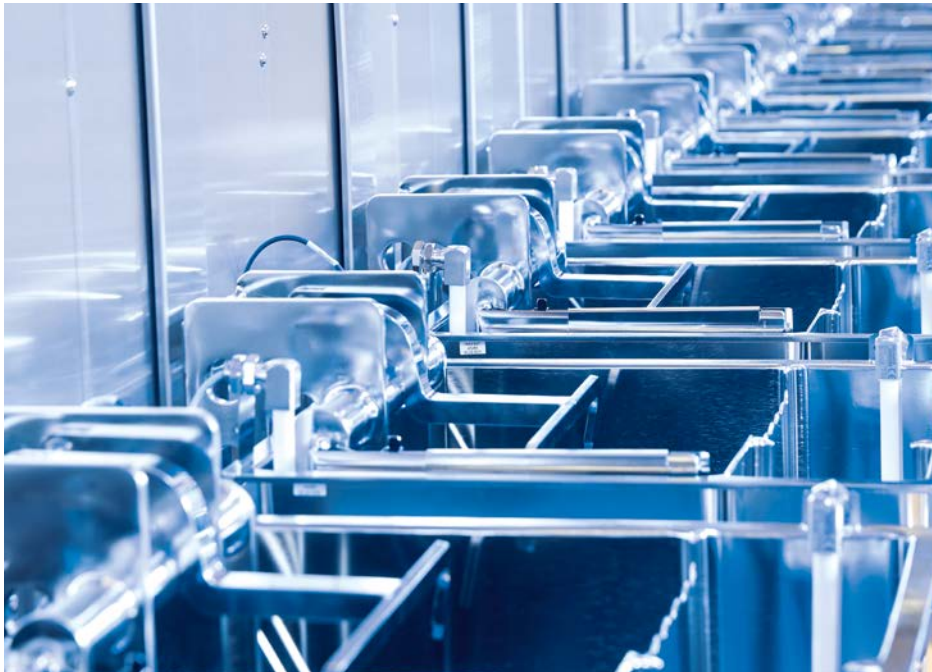
MEDLINE – View into process chamber for cleaning and deposition of daily lenses.
