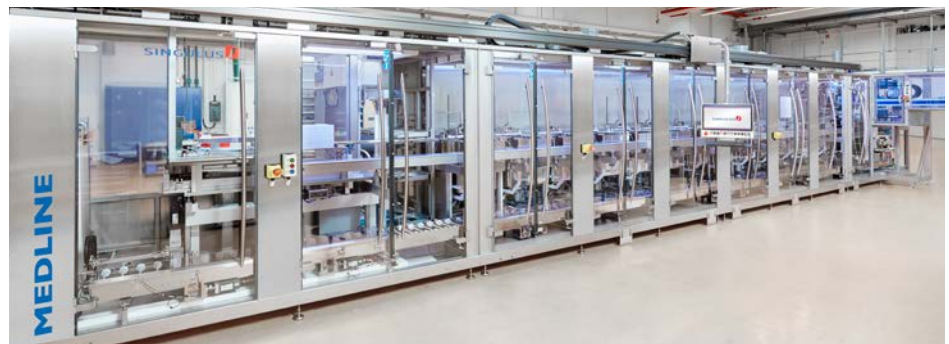
DECOLINE II: Manufacturing line for sustainable coating of 3-dimensional parts. This manufacturing solution is interesting for automotive, consumer goods, sanitary parts, mobile phones and packaging used in the cosmetics or beverage industry. Decorative coatings will address many new applications.
