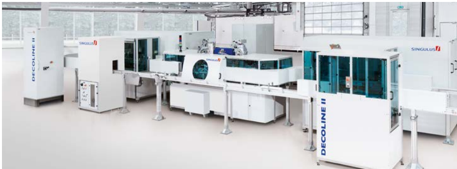
DECOLINE II: Manufacturing line for sustainable coating of 3-dimensional parts. This manufacturing solution is interesting for automotive, consumer goods, sanitary parts, mobile phones and packaging used in the cosmetics or beverage industry. Decorative coatings will address many new applications.
