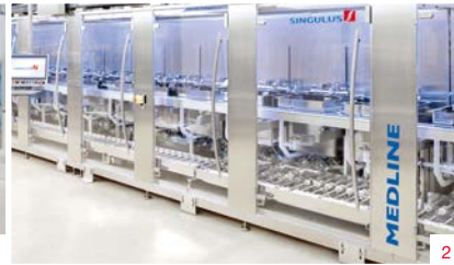
2: Large inline sputtering with vertical substrate transport
