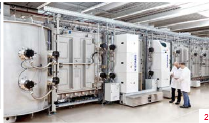
2: Large inline sputtering with vertical substrate transport
