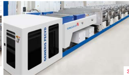
3: PECVD inline system for high-performance solar cells
