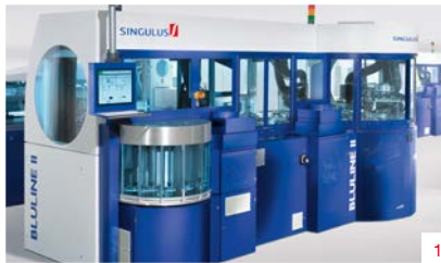
1: BLULINE replication line for production of writable discs for data storage applications
