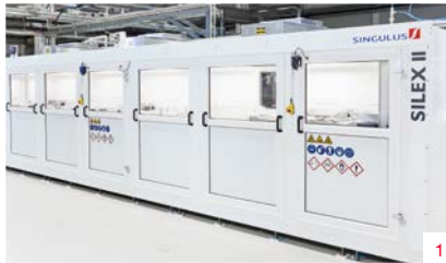
1: SILEX II wet processing system
