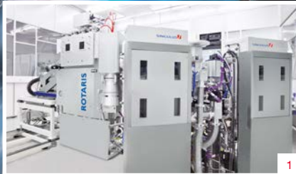
1: ROTARIS R&D and pilot system for vacuum deposition
