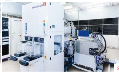
2: TIMARIS II ultra-high vacuum deposition system
