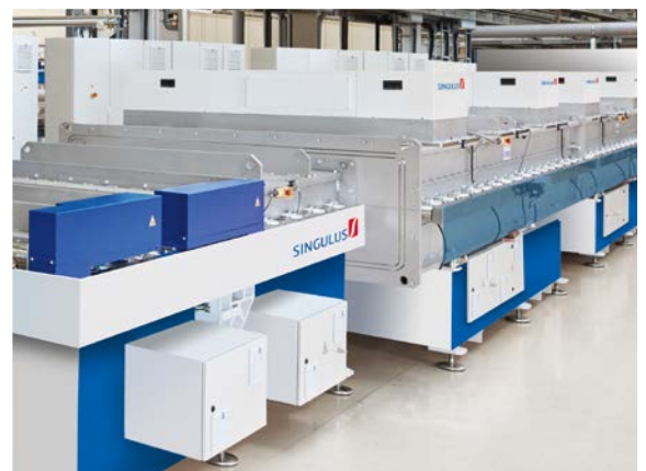
Inline Sputtering System with Horizontal Substrate Transport for Flat Substrates
